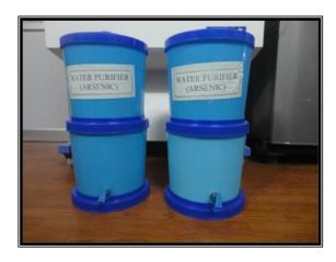
Water filtration system for removal of fluoride and arsenic (Domestic model – 15 L capacity) has been developed which has arsenic removal efficiency of 87 % and Fluoride removal efficiency of 92 %. The Cost of the model is Rs. 1000.00. The model has been installed at Government school, Mavinamatti, Shahapur, Yadgir (Dist.) in collaboration with IIT, Chennai for removal of arsenic from drinking water.
